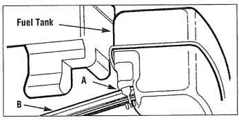
Figure 31: Hose clamp and fuel line.
